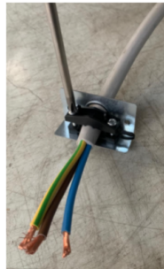
Fix power cord to the plastic holder.
